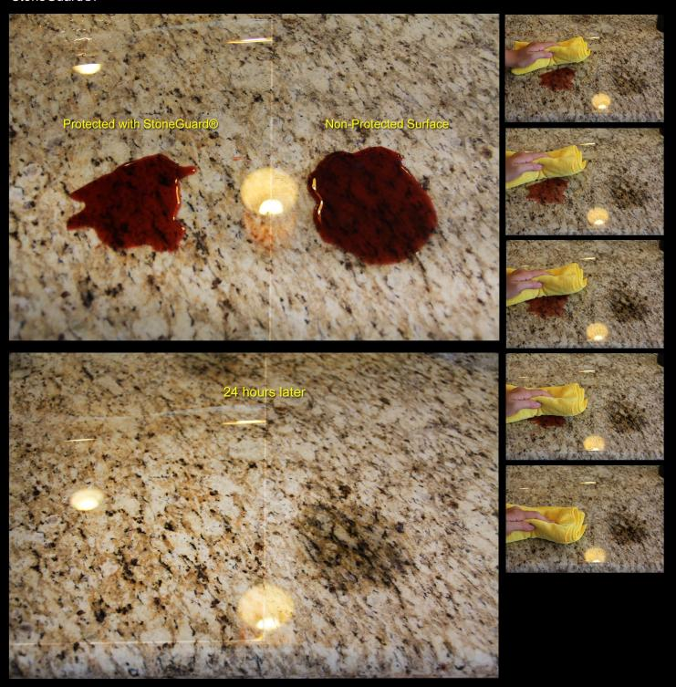
Image above illustrates staining on the unprotected stone surface from red wine.
